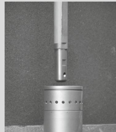
For shot blasting the internal surface of cylindrical components we offer specially designed internal blast nozzles connected to a pressure blast system. We will be happy to assist you with your shot blasting challenges.
