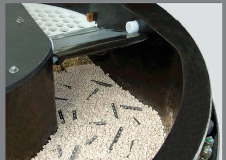
Pneumatically activated separation flap
