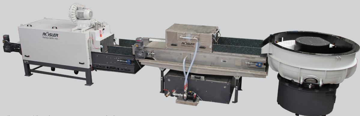
Rotary vibrator with subsequent conveyor belt washing installation and hot air belt dryer
