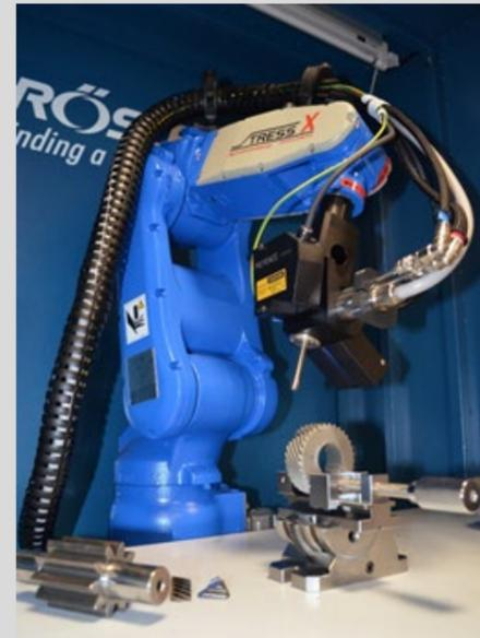
Besides our in-house x-ray diffractometer we also utilize suitable electropolishing and measuring technologies to document the compressive residual stress curves.
