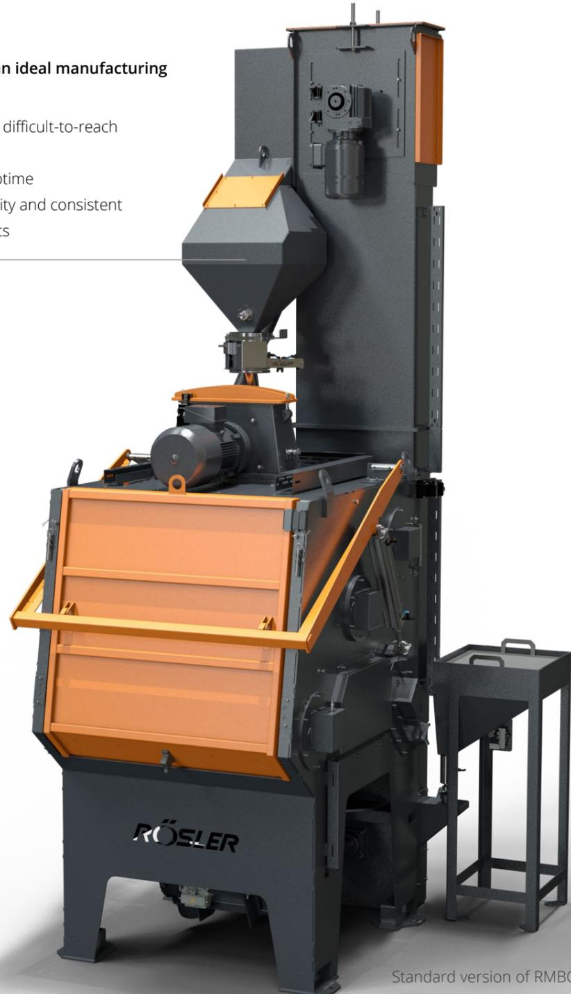
Standard version of RMBC HD for manual work piece loading/unloading; equipped with media replenishment system
