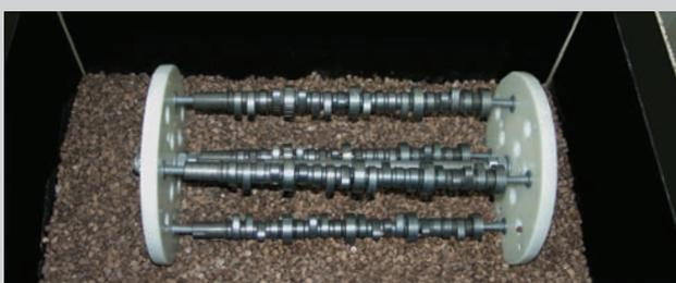
To prevent part-on-part contact, multiple delicate work pieces can be mounted to a special fixture.
