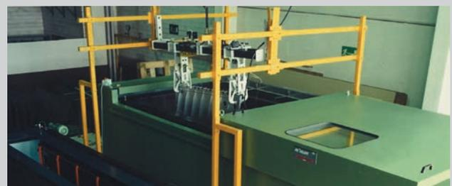
Loading and removal of high value work pieces into and from the work bowl with custom engineered handling systems.
