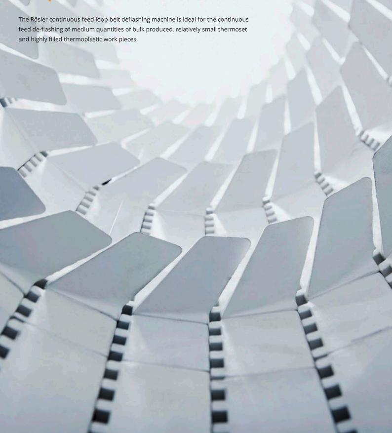
The raw work pieces are transferred into the de-flashing machine by an angled belt conveyor in combination with a vibratory feed chute. The rubber loop belt is equipped with cams that are arranged in an auger-like fashion. While the work pieces are constantly tumbling over each other, the cams are gently pushing them forward through the blasting zone at a preset speed. The RSBS is equipped with two blast turbines placed in the roof of the machine housing above the loop belt.
