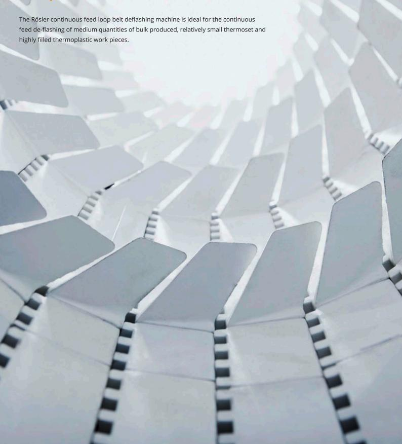
The raw work pieces are transferred into the de-flashing machine by an angled belt conveyor in combination with a vibratory feed chute. The rubber loop belt is equipped with cams that are arranged in an auger-like fashion. While the work pieces are constantly tumbling over each other, the cams are gently pushing them forward through the blasting zone at a preset speed. The RSBS is equipped with one blast turbine placed in the roof of the machine housing above the loop belt.
