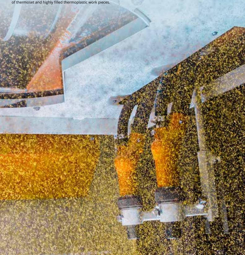
The rotary system, consisting of two firmly connected satellite tables with their own rotary drive, allows the de-flashing of single or multiple parts on one table, while finished parts are removed and raw parts loaded at the other table. By a 180° system rotation the satellite tables move from the blast zone into the load / unload zone and vice versa. Depending on their size, up to eight work pieces can be placed on each satellite table.
