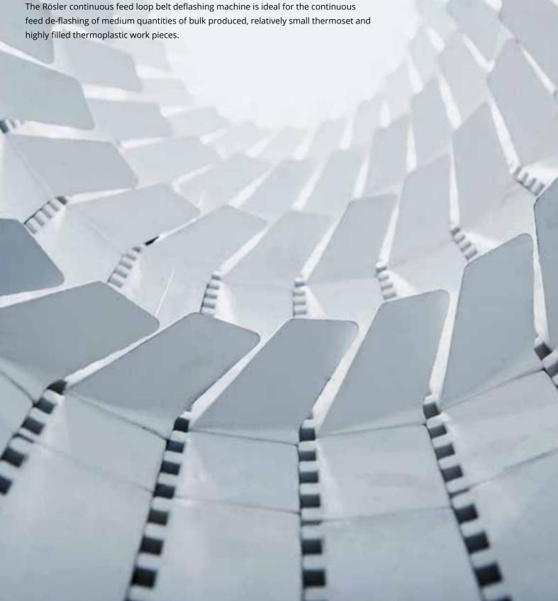
The raw work pieces are transferred into the de-flashing machine by an angled belt conveyor in combination with a vibratory feed chute. The rubber loop belt is equipped with cams that are arranged in an auger-like fashion. While the work pieces are constantly tumbling over each other, the cams are gently pushing them forward through the blasting zone at a preset speed. The RSBS is equipped with one blast turbine placed in the roof of the machine housing above the loop belt.
