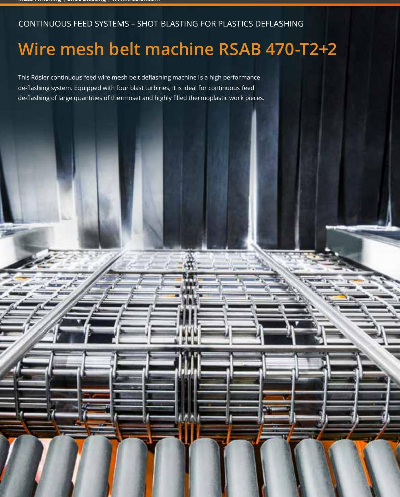
Four blast turbines – two placed above and two placed below the wire mesh belt – produce a highly intensive de-flashing process with uniform finishing results. After the turbines have thrown the blast media, a bucket elevator transports it to a cascade air wash separator located above the turbines removing dust and other contaminants from the media.
