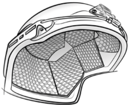
Helmet padding with a micro lattice structure
